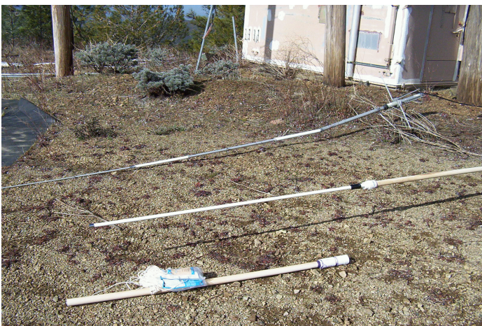
The CX-333 antenna with the bottom PVC section in place, the top section is in the foreground. The white and blue stuff is the coiled up guy cord.
